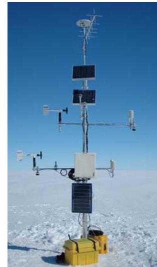
NSF AWS with GPS, net radiation sensor and two sets of wind, temperature and humidity sensors spaced one metre apart. Three identical stations were installed on Larsen C this season.
